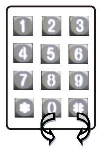
Press 0# simultaneously, LCD screen will stop scrolling if the LCD is still scrolling repeat the process then 4-digit Master Code (0000 is default master code)
